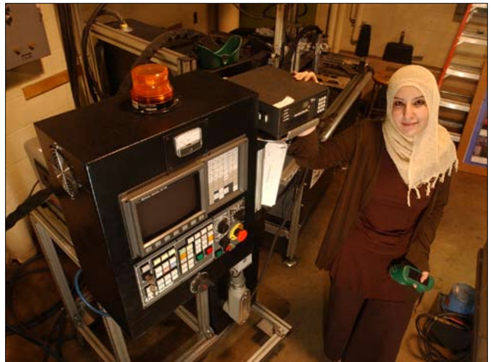
AN ENGINEER'S TOUCH – Newly-minted computer engineer Manar Wadi poses with the controller she adapted to run a plasma cutter in mechanical engineering laboratory. The senior project capped four years of hard work at Lake Superior State for Wadi, who started with a telecommunications company this fall in her home town of East Jerusalem.
