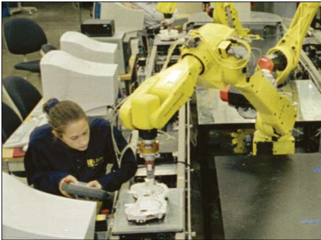
Karel software is used to program a family of Fanuc Arcmate robots.
