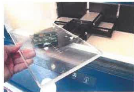
Standard quick-change stage interface for easy placement of a sample outside the sample chamber.
