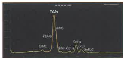
Peaks of Pb and Bi Specimen: Wood metal
