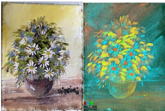
Visual (right) versus \mu XRF imaging of a painting (circa 1969). Chemical composition is visible via \mu XRF: sulfur (red), titanium (blue),
